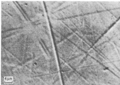
Figure 7 Scanning electron micrograph of the articular surface of the acetabular component removed from Patient 2. Note the broad scratches resulting from corrosion.
