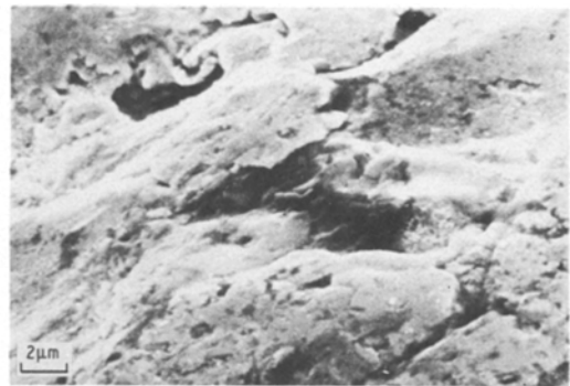
Figure 8 Scanning electron micrograph of the pelvic surface of the acetabular component of the prosthesis removed from Patient 3. Note the irregular surface resulting from corrosion.
